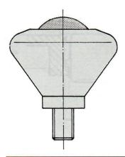
bulb-shaped with threaded bolt
